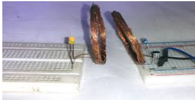
Fig 5: Wireless Power Transmission between Coils
